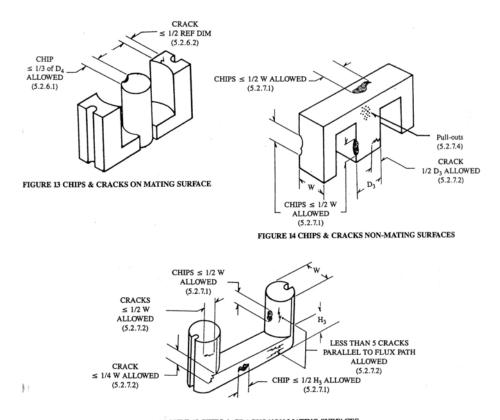
FIGURE 15 CHIPS & CRACKS NON-MATING SURFACES
