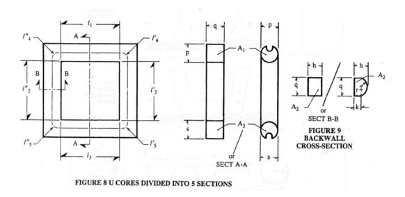
Path lengths  $I_1 & I_3$  associated with  $AI_1 & I_3$  as shown. Length of flux path associated with area  $AI_2$  is:
