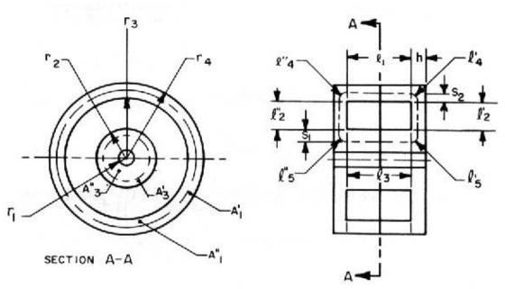
FIGURE 6 POT CORE SET DIVIDED INTO 5 SECTIONS
